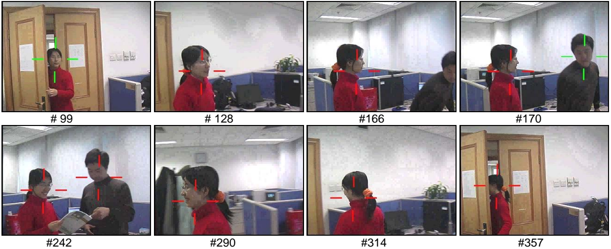
Figure 4. A sequence of two interacting persons tracking in indoor environment with an active camera. Note that serious problems as heavy rotation (Figure 4, frame #166, frame #170, frame #314, frame #357), scale changes (Figure 4, frame #99 and frame #290) and changing background are correctly handled.
