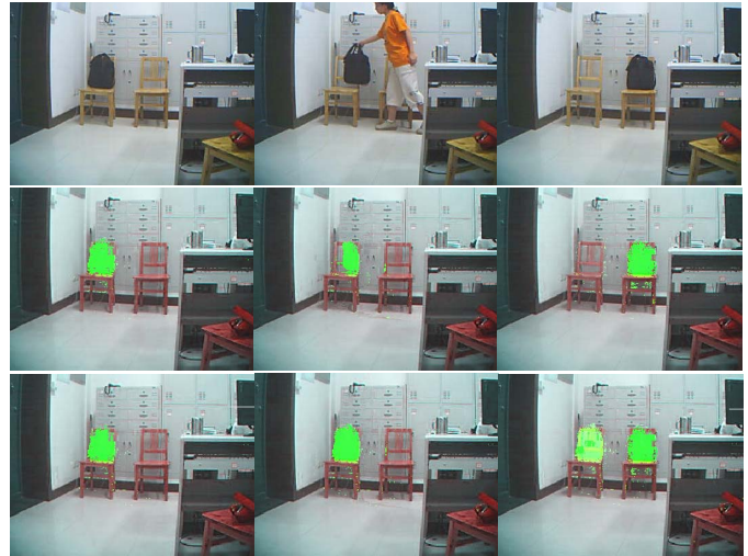
Figure 4. Abandon object detection. These images are captured at frame #262, frame#432, frame#541. The first row contains the input video. The second row contains the abandon object detection result of our method. The third row contains the detection result without multiple background layer. The green area represents the abandon object.
