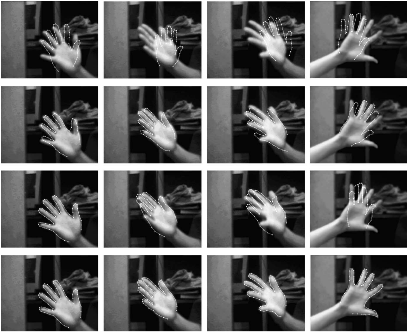
Fig. 4. Comparison of the three methods. Top: initial. Second row: Tracking results of AI-Snake. Third row: Results of ASM. Last row: Results of the proposed AI-ES.
