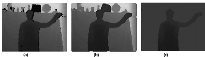
Fig. 3. It shows the results by the preprocessing step. (a) original frame, (b) image smoothing, (c) background removal. The image is derived from [33].
