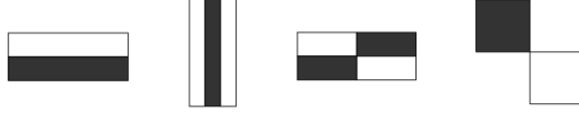
Fig. 1. Traditional Haar-like features. These features measure the differences between rectangular regions' average intensities
