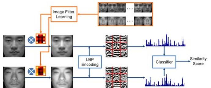
Figure 2. The pipeline of face representation and recognition with image filter learning based descriptor.
