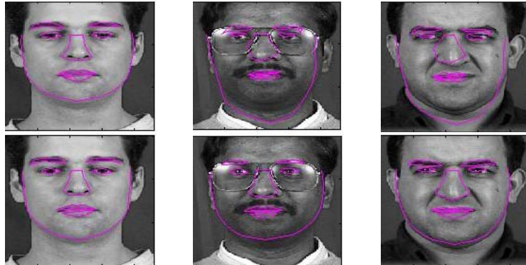
Fig. 6. Comparison results of ASM and GCASM with Bayesian inference. The first row is ASM results, and the second row is our results.
