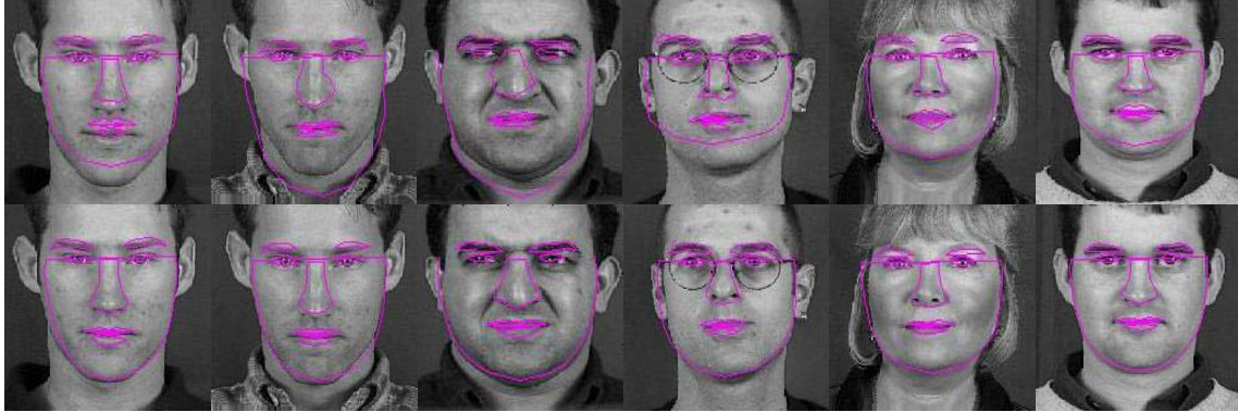
Figure 4: Comparison results of ASM and our method. The first row is ASM results, and the second row is R-ASM's results.
