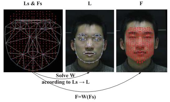
Fig. 3. The warping process of facial points. Left: Standard landmarks  $L_s$  (blue dots) and facial points  $F_s$  (red dots). Middle: A face image and its corresponding landmarks  $L$ . Right: the warped facial points  $F$  for the input image.
