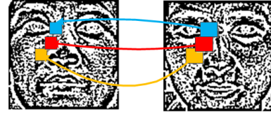
Figure 5. NIR-VIS face image matching strategy for BLoG. The 256 \times 320 pixel area of a face is divided into 16 \times 16 local patches.
