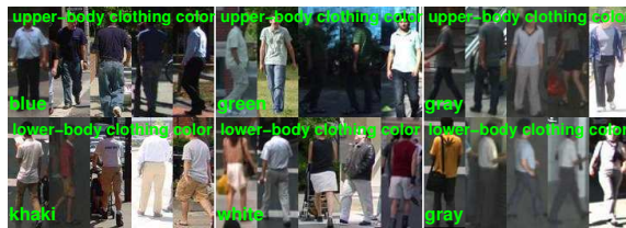
Figure 7. Some samples that are difficult to be classified in multi-class attribute classification. Many mis-classified classified blue samples are dark blue and light blue samples. Results are affected by illumination condition ( green , gray ), large background between legs ( khaki ) and short clothing length ( white ).
